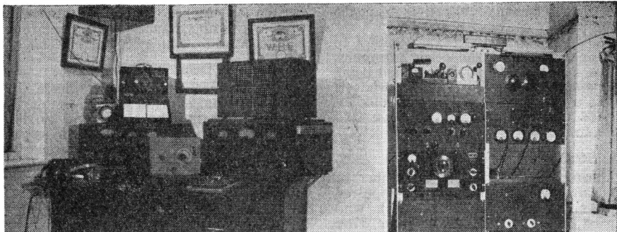
The outfit at G5PY, Clapham Park, London, an active 5-metre station. The Rx side comprises an S27 for general VHF listening, with an EF54-EF50-EC52 converter into an SX28 at 8.5 mc for 50 and 58 mc reception. The transmitter, power supply and modulator complete are carried in the rack assembly, the 58 mc PA being an 807 FD ; this is shortly to be replaced by a pair of RK34's to "reach 144 and 420 mc." G5PY's aerial is a 3-element rotary beam, controllable from the operating position.
